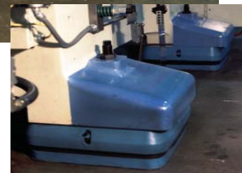
Installation of a high-speed press on VSML Isolators
